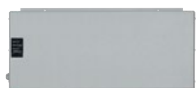
UPS system For bridging power failures of up to 2 hours and up to 4 door cycles; safety devices, warning lights, etc. remain functional, LED status display, automatic battery test, surge filter, protection category: IP 20 Dimensions: 560 x 235 x 260 mm (W x H x D)
